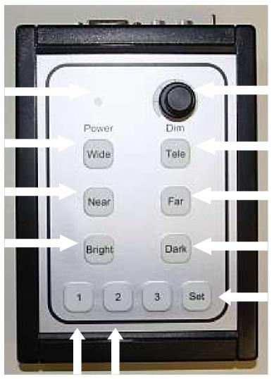
The buttons 1 and 2 are memory buttons, 2 different camera settings can be stored and recalled.
