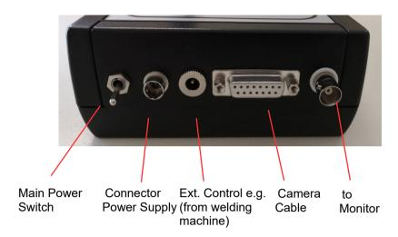
At the back of the operating device are the connection of the power supply, the 15 pin Sub D socket for the connection of the camera cable, a connection for external control of the special filter and a connector to the Monitor.
